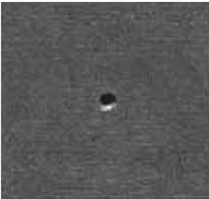
Detail of an identified defect: hole
