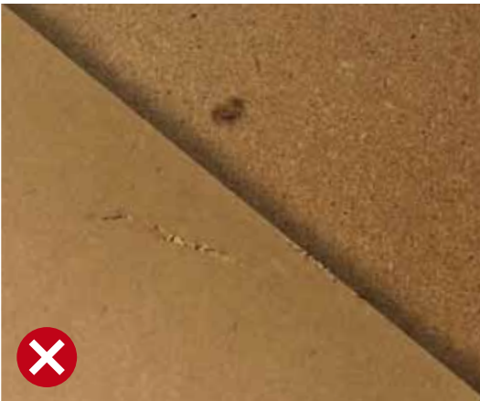
Faulty raw panel quality, bottom MDF, top particleboard
